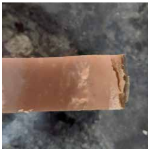
Overheating and cracking on edges.
